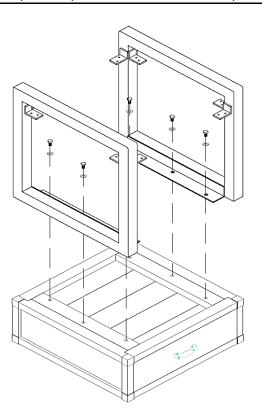
Attach the legs using bolt (A) and washer (B).
