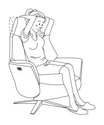
To adjust the headrest, grip the backside of the headrest and pull forward from both sides as shown
