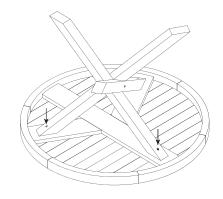
• Step 1: Join L1 and L2 together using bolts and washers, tighten the bolt by <a href="https://hand.only.">hand only.</a>
