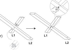
• Step 2: Join the 3<sup>rd</sup> leg using bolts & washers, tighten the bolts by hand only. Make sure the concave of L2 match with the edge of L3, and L3 with L1 are similar, all creating 90° angle.
