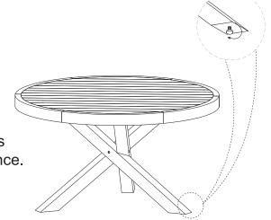
• Step 6: Turn the table over. Adjust the rubber pin under each leg untill each rubber pin touches the ground, so that your table will be in balance.
