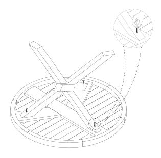
• **Step 5:** After the 3 legs are in their correct position, tighten the bolts at the legs<sup>(1)</sup> and the top section<sup>(2)</sup> with hex key.
