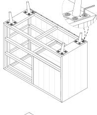
• Step 4: Turn the cabinet over, then adjust the rubber pin under each leg untill each rubber pin touch the ground, so that your cabinet will be in balance.
