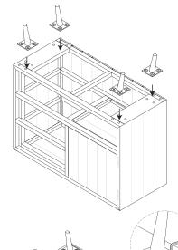
• Step 3: Fit the 4 angle legs to the cabinet's corner locations by using bolts and washers.
