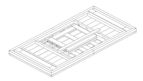
STEP 1 We suggest to place the table upside down on a blanket to protect it from scratching. Unlock locking clips
