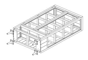
• Step 3: Fit the 4 angle legs to the cabinet's corner locations by using bolts and washers.
