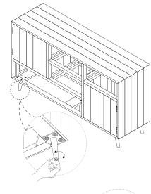
Step 6: Insert the drawers and turn the drawer stops up to prevent the drawers from falling out when you open.
