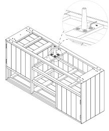
• Step 4: Fit the 4 angle legs to the cabinet's corner locations by using bolts and washers.
