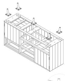
• Step 3: Fit the straight leg to the centre location. Insert all 4 bolts with washers into their slots, then tighten the bolts by using the hex key provided.
